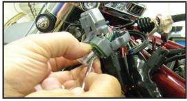
3. Locate pins 20 and 16 (unused in the current configuration), and remove the seal pin plugs. Insert the terminated black wire into pin 20, and the red wire into pin 16 on the "wire side" of the connector.
